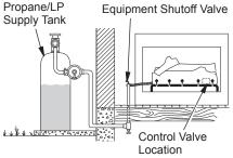
Figure 15 - Checking Gas Joints (Propane/LP Gas Only)
